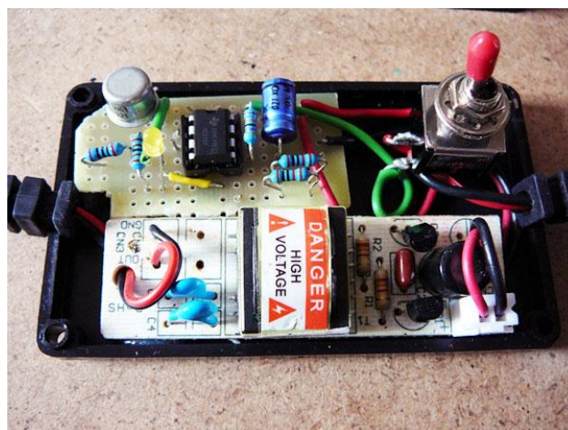
Fig.6: The inverter with timer for the Xenon calibration tube
