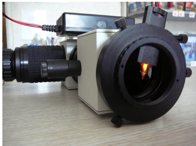
Fig.2: The Neon calibration unit in a holder that can be easily pulled out or inserted in the ring attached to the DADOS.
