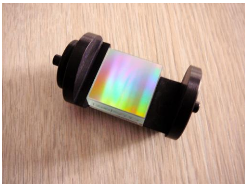
Fig.1: 1200 l/mm grating in its holder
